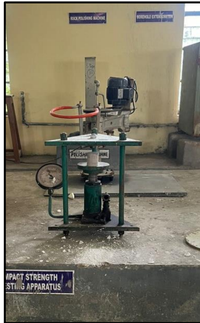
Fig 3.9 Point Load Index tester
