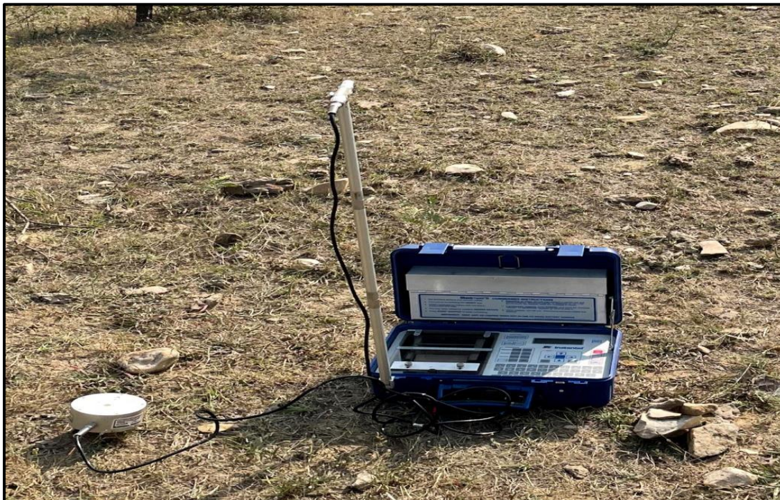
Figure 3.6 Instruments used in ground vibration measurements
