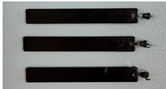
Fig 6: Tensile and impact sample prepared by micro injection moulding machine according to ASTM standard
