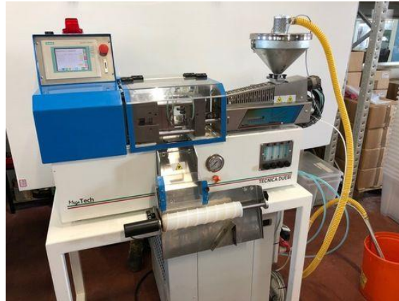
Fig 5: Micro injection moulding machine
