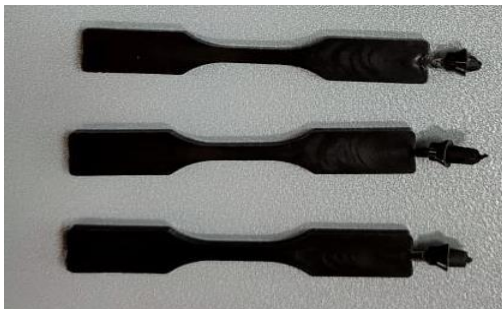
Fig 6: Tensile and impact sample prepared by micro injection moulding machine according to ASTM standard
