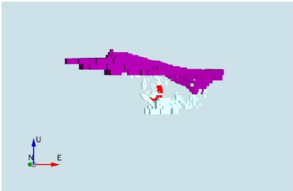
Figure 1: A Figure showing the designed stopes within the IMAT model, Vertical Projection, North Orientation
