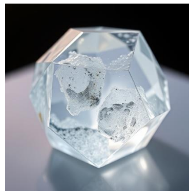
Fig-1 (b) As grown crystal of 1 mole % KI doped ZTS
