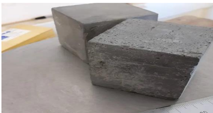
Fig 2 concrete cubes after de-moulding
