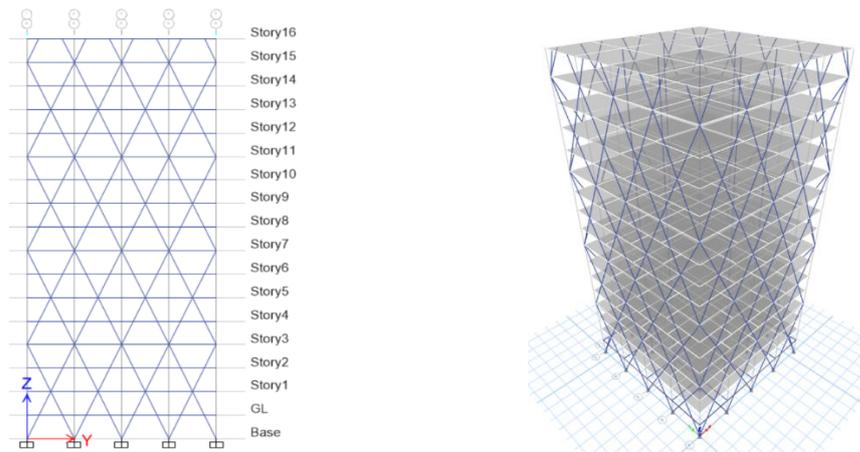
**Figure 9 – Elevation and 3D View of Diagrid Frame Structure Model 5 with angle as 64.88°.**
