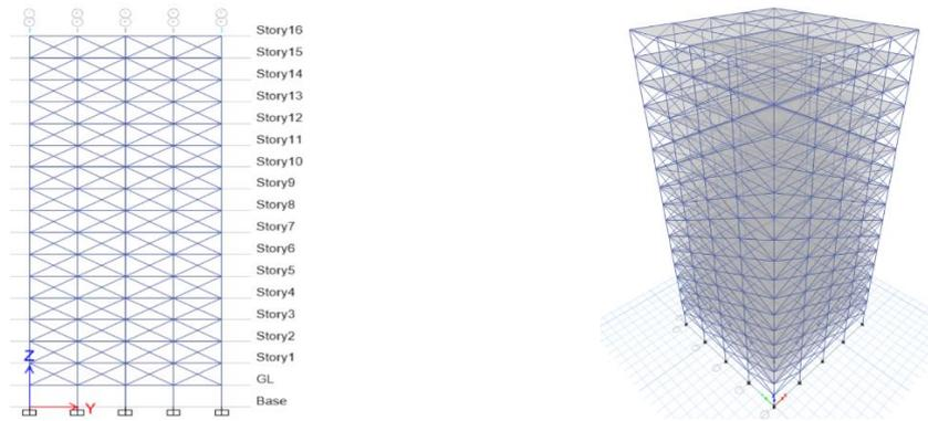
**Figure 6 – Elevation and 3D View of Braced Frame building Model 2**
