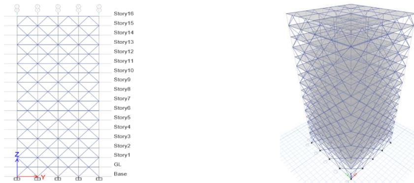
**Figure 7 – Elevation and 3D View of Diagrid Frame Structure Model 3 with angle as 46.84°.**
