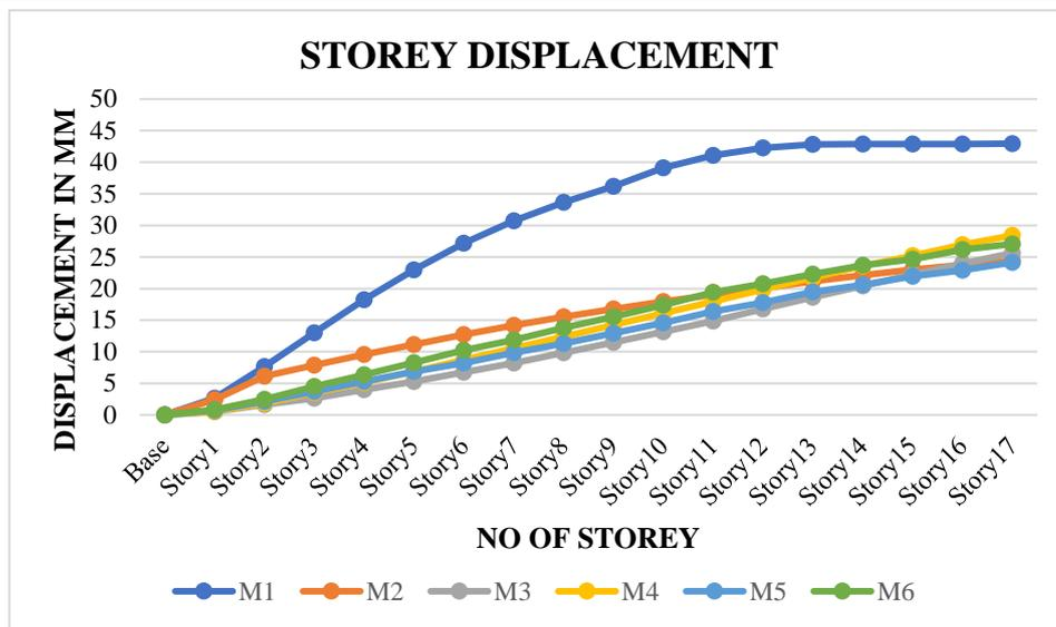
Graph 1: Displacement in mm due to time history analysis for all models along x & y-direction
