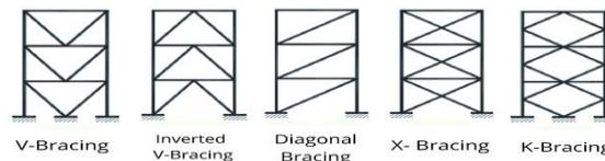
**Figure 2 - Types of Bracing Structural System**
