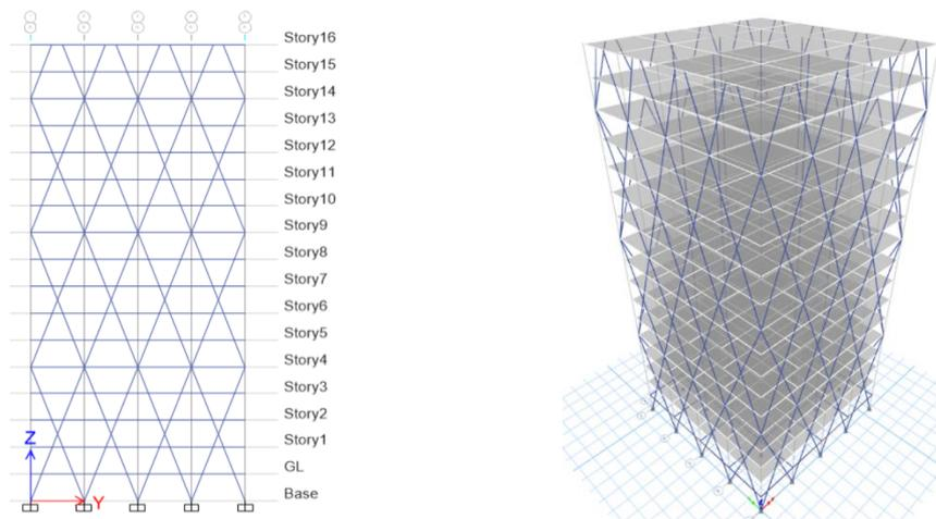
**Figure 10 – Elevation and 3D View of Diagrid Frame Structure Model 6 with angle as 69.44°.**
