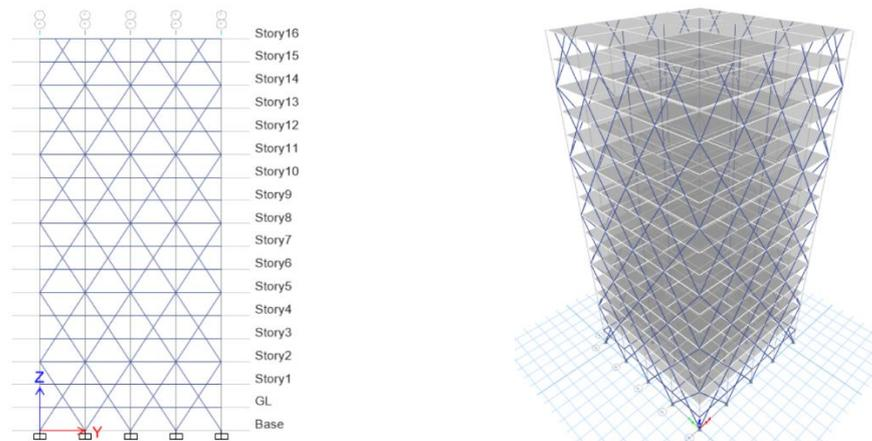
**Figure 8 – Elevation and 3D View of Diagrid Frame Structure Model 4 with angle as 57.99°.**
