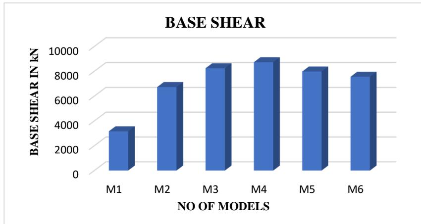
**Graph 3: Base shear in kN for all models in the x and y directions by time history analysis.**
