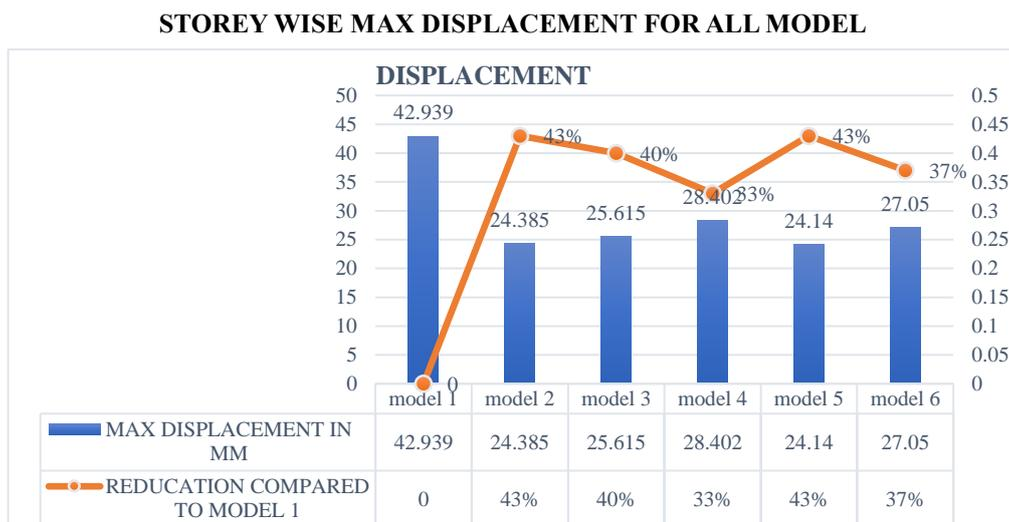
According to the graph, model M1 has the most displacement compared to any model. The bracing system was used for the RC frame building in model M2, which resulted in a displacement reduction of 43.21% as compared to M1. The displacement in the model M5 is reduced by 43.78% in comparison to the M1 due to the existence of a diagrid frame structure and is almost the same for the M2 bracing system.
