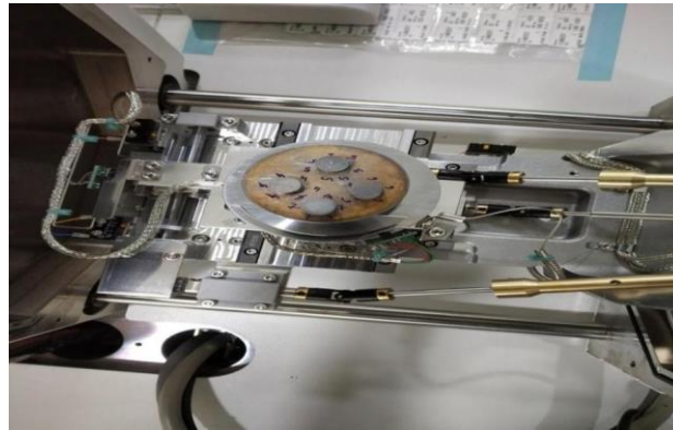
Figure 14: Placement of samples in the machine for SEM and EDX study
