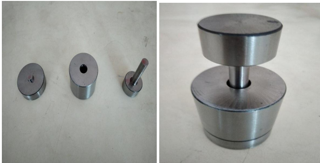
Figure 6: Punch and die used for compression of powder
