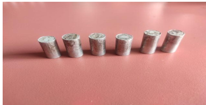
Figure 12: Sintered cylindrical specimens with different weight percentage of reinforcements
