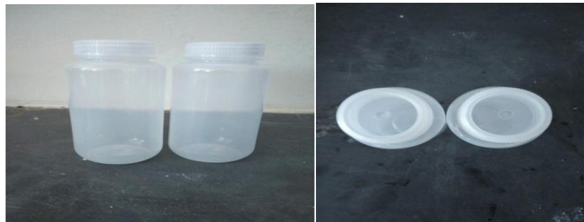
Figure 5: Polypropylene bottles used for milling and mixing of powders
