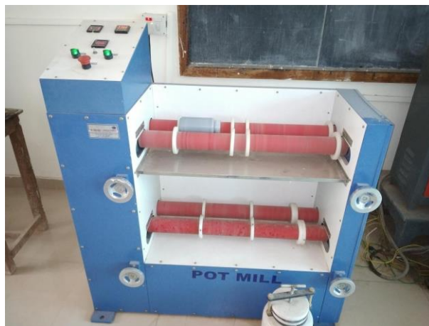
Figure 4: Pot mill used for milling and mixing of powders
