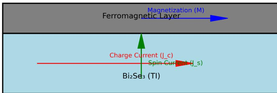
**Figure 2: TI-Based Spintronic Device**
