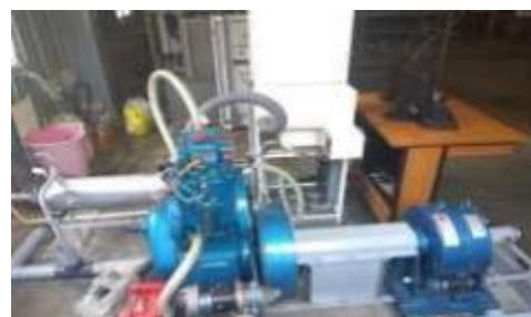
Fig.4 Side view of VCR 4-stroke diesel engine
