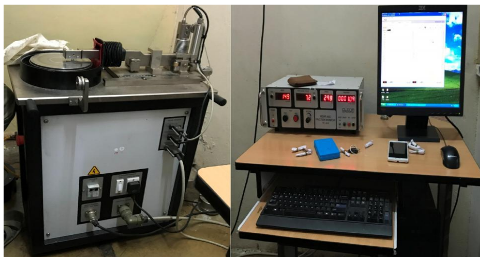
Figure 9: Experimental set up of wear test
