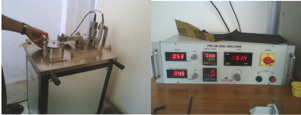
Fig. : 7(a) Pin on disc wear testing machine, (b) Display unit
