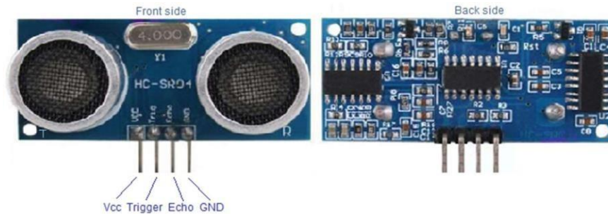
Fig 4.1.11 Pin Description and View of Ultrasonic Sensor VCC: 5V DC supply voltage is connected to this pin.
