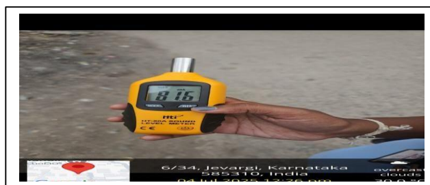
Fig.No.4.Monitoring of Noise level in Residential Area
