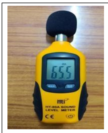
Fig.No.3.Representing the Sound level meter to measure Noise pollution of Jewargi town
