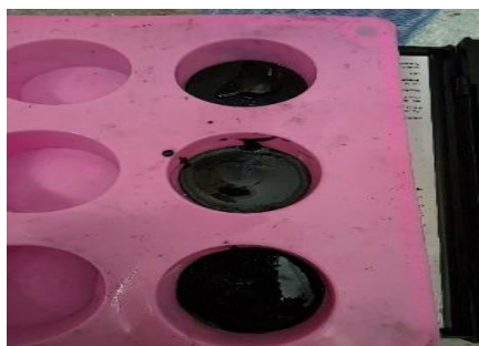
Figure 8: Casting of CNT/Epoxy Nanocomposites into Molds
