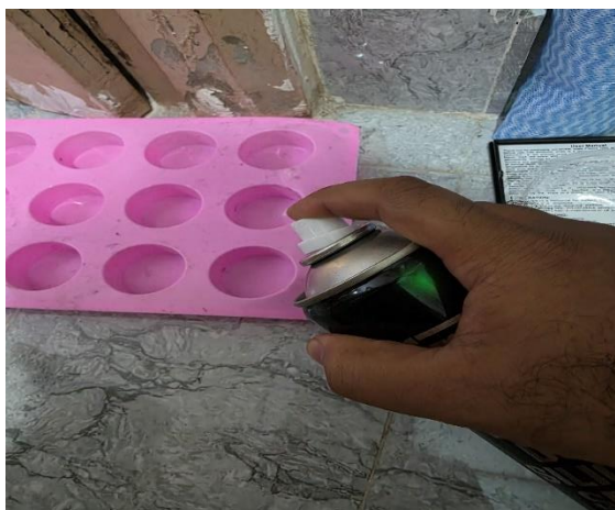
Figure 7: Application of Release Agent to Mold
