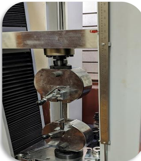
FIGURE 10: RECORDING THE CHANGE IN LENGTH
