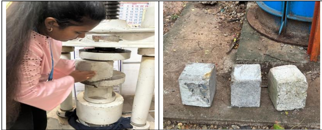
Figure No. 9: Compressive Testing of Cubes
