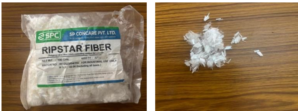
Figure No. 4: Polypropylene Fibre from SP Concure Pvt. Ltd. was used
