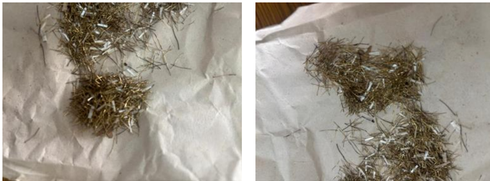
Figure No. 3: Micro Steel Fibre was used in present investigation
