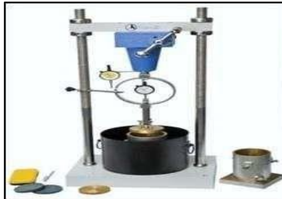
Figure No. 6: Swell Pressure Test by Volume Method
