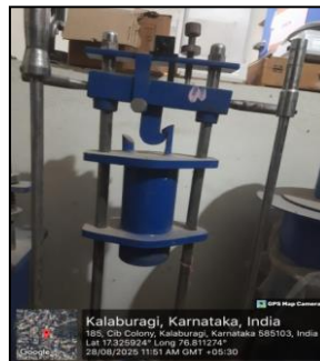
Figure No. 6: Impact Value Test at Laboratory
