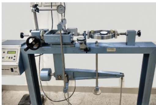
Figure No. 4: Direct Shear Test at Laboratory
