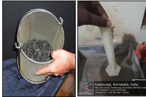
Figure No. 5: Specific Gravity Wire Basket Test at Laboratory
