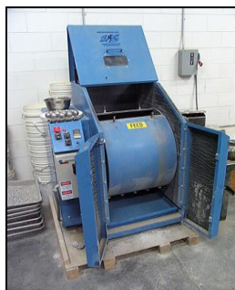
Figure No. 8: Abrasion Test at Laboratory
