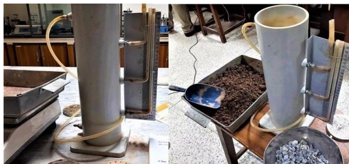
Figure No. 9 Permeability Test at Laboratory
