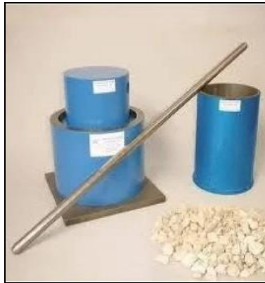
Figure No. 7: Crushing Value Test at Laboratory
