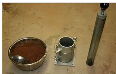
Figure No. 10: Modified Proctor Test at Laboratory
