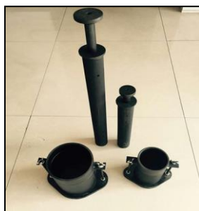
Figure No. 3: Proctor Compaction Test at Laboratory
