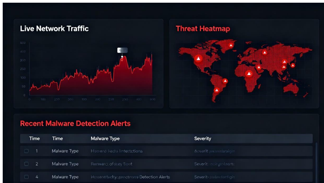
Figure 4: Real-Time Dashboard Screenshot shows the web interface displaying live traffic, threat heatmap, and recent alerts. The system auto-generates daily CSV reports with detection statistics.
