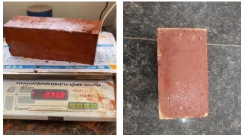
Fig 6.2: Brick density of red mud brick
