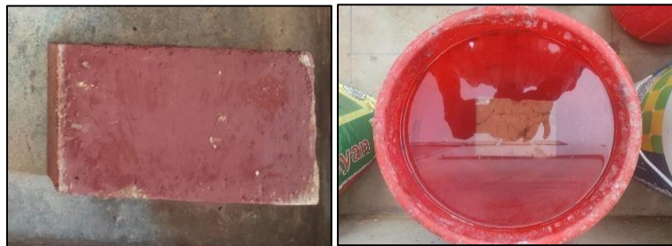
Fig 6.3: Water absorption test on masonry unit
