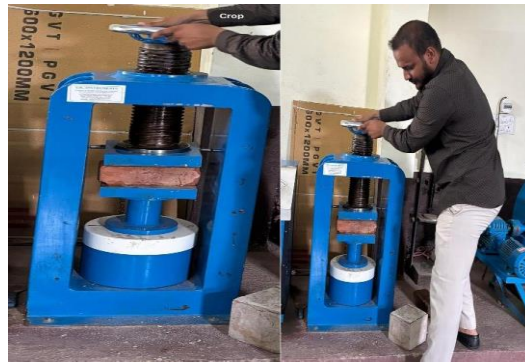
Fig 6.4: Compression Test on Red mud bricks
