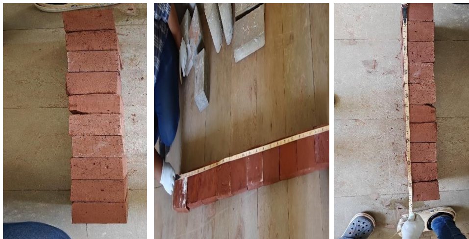
Fig 6.1: Dimensionality Test of Red Mud Bricks
