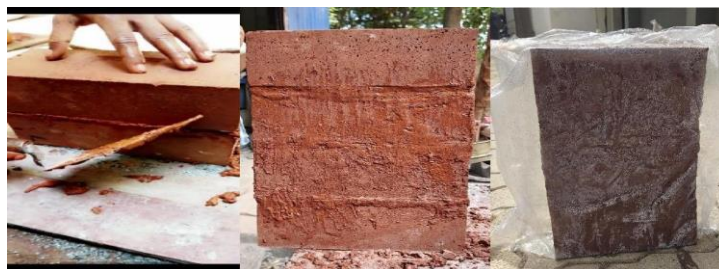
Fig 6.8: Casting And Curing of Prism and Triplet
