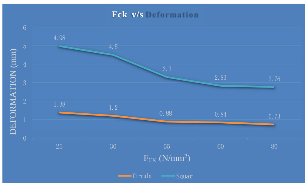
Fig 4.5: Grade X Deformation Graph of Concrete
