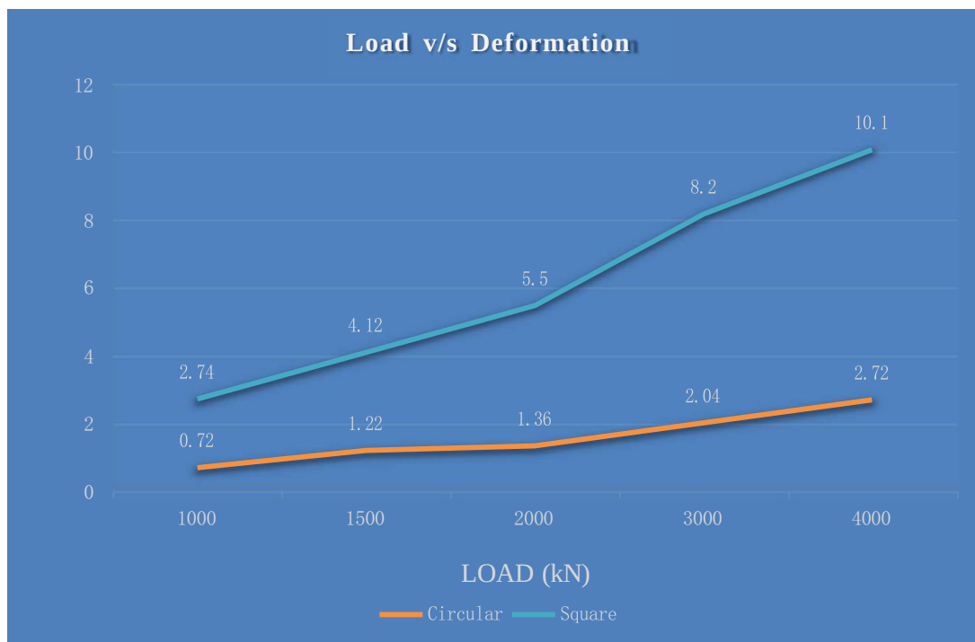
Fig 4.3: Cement Column Deformation Behavior
