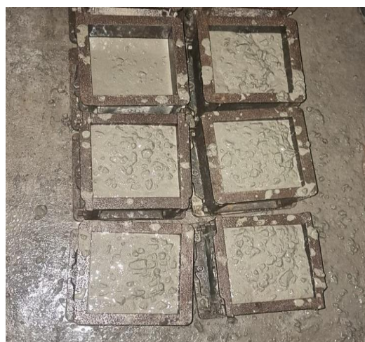
Fig No 5.1: Casting of Cubes
