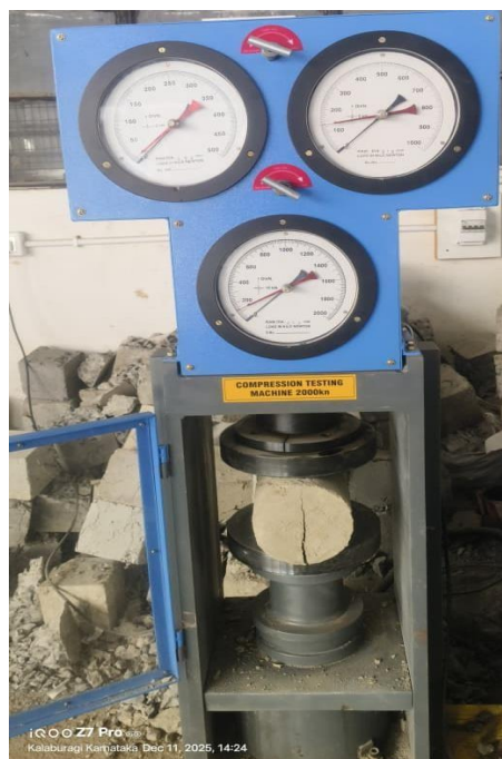
Figure 6.2.1: Split Tensile Strength
