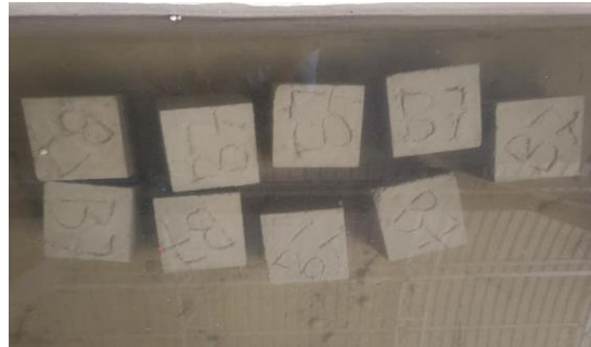
Fig 5.4.1: Curing of Cubes in Water
