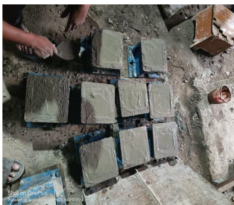
Fig 5.3: Casting of Specimen
