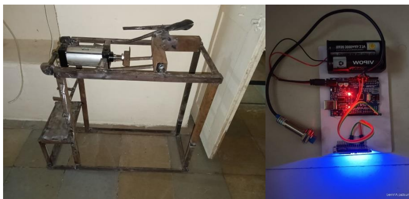
Figure-2: Automated Pneumatic Sheet Metal Cutting & Crushing System with Sensor-Based Counting
