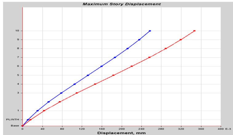
Graph 13:-Storey v/s storey displacement of building with concrete blocks infill walls without opening
