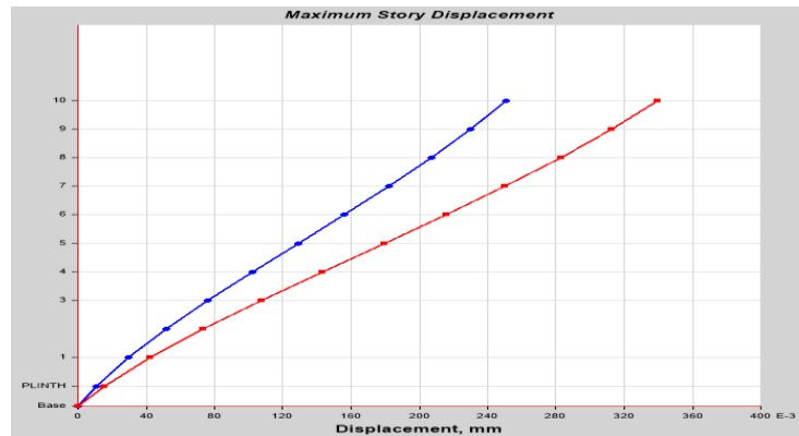
Graph 9:- storey v/s storey displacement of building with brick infill walls without opening
