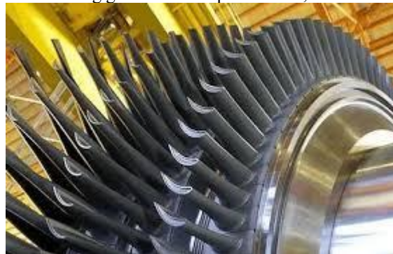
Figure 29. actual blade design used in steam turbines for 1-2 kw
