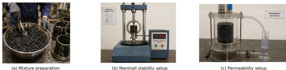
Figure 2. Mixture preparation, Marshall stability apparatus, and permeability apparatus reproduced from the thesis.
