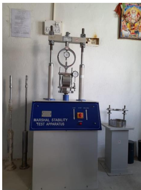
Figure 3. Marshall stability testing machine used in the experimental programme.
