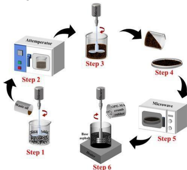
Figure 2. Wet-process preparation sequence reported in the thesis.
