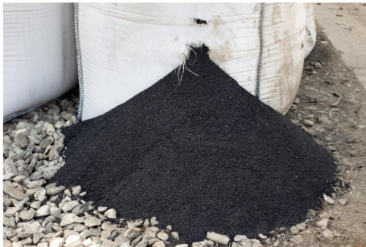
Figure 1. Crumb rubber used for bitumen modification, reproduced from the thesis.
