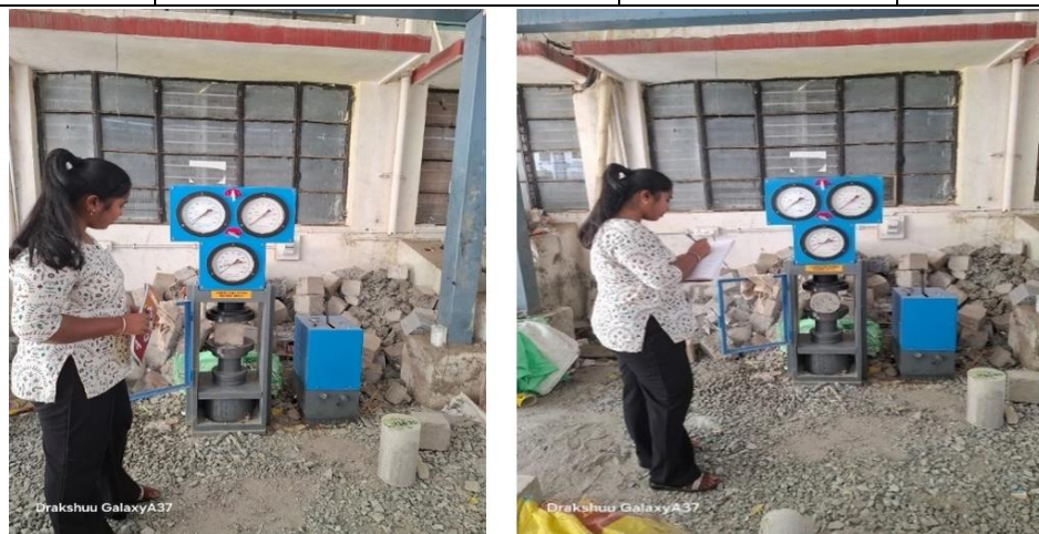
Fig. 2. Compressive-strength and split-tensile-strength test arrangements reported in the thesis.
