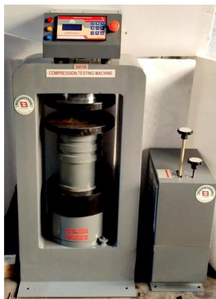
Fig. 1. Compressive-strength testing machine retained from the thesis.
