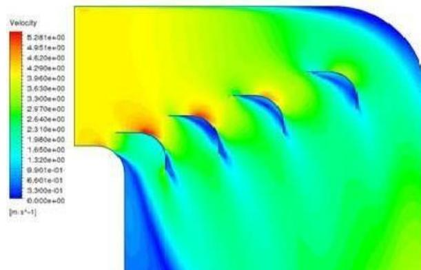
**Fig 10 : Velocity Contour with vanes**
