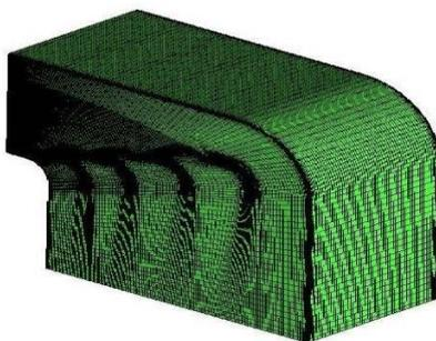
**Fig. 3 : Mesh for ducts & vanes**
