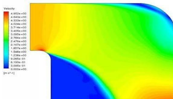
**Fig. 8: Velocity Contour without vanes**
