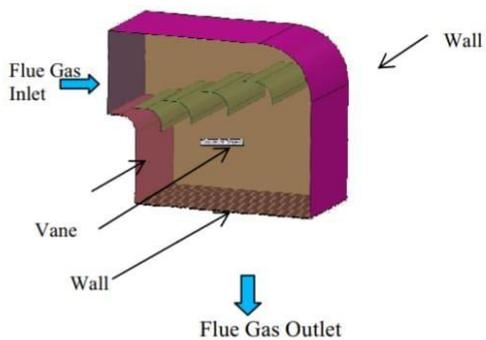
**Fig 2 : Inlet duct geometry with vanes**
