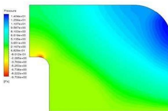
**Fig.14 : Pressure Co n t o u r without vanes**
