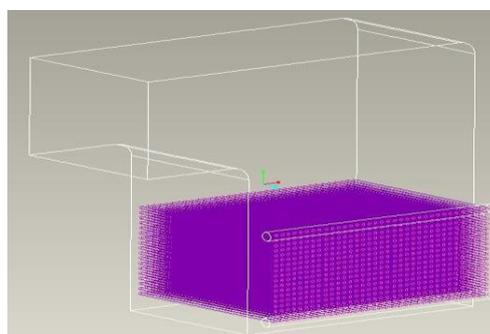
**Fig. 1 : Geometry of inlet duct & Economizer**
