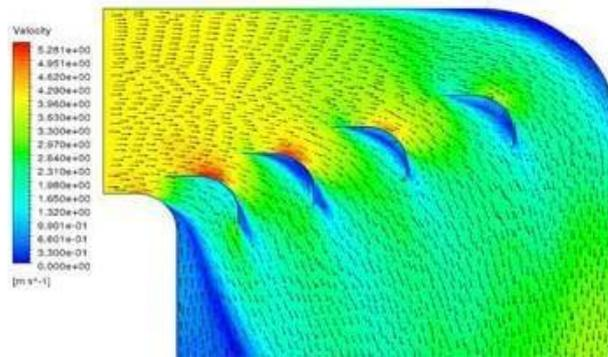
**Fig.13 : Velocity Vector with vanes**
