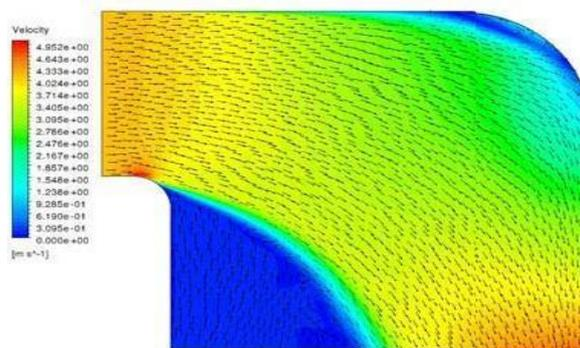
**Fig 9: Velocity Vector with no vanes**
