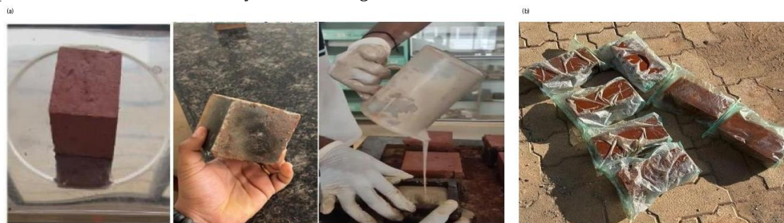
Fig. 1. Specimen casting and moisture-retaining thermal curing.
