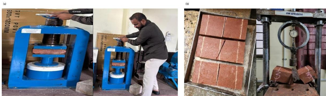
Fig. 2. Experimental arrangements for brick compression and flexural testing.
