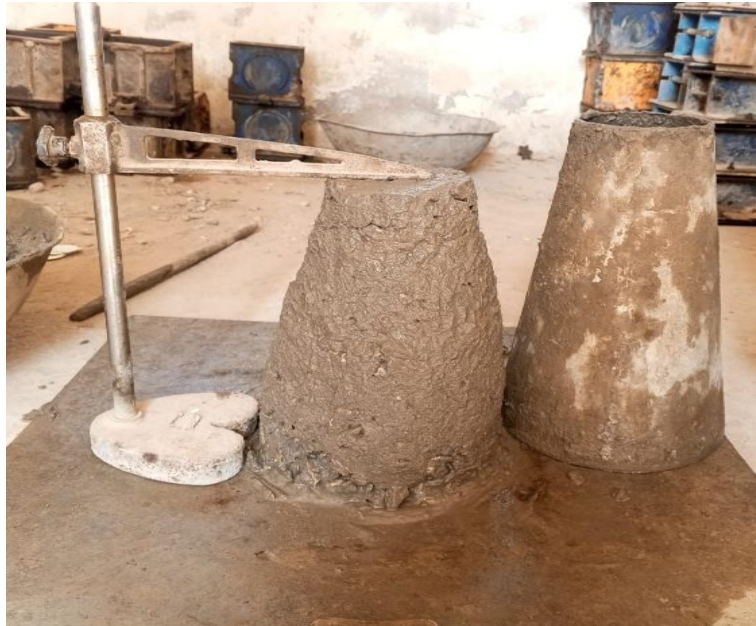
Figure 3. Workability of fresh concrete setup.
