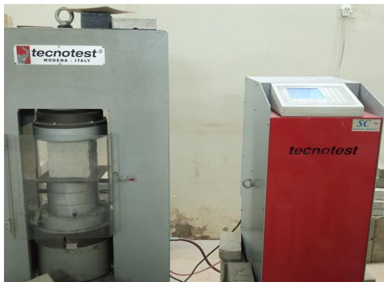
Figure 4. Testing of cubes under universal testing machine.
