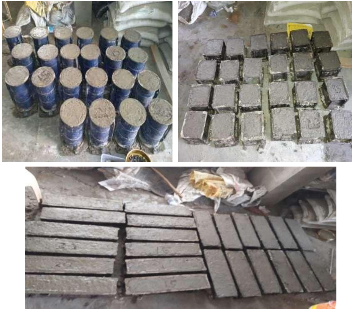
Fig 4: Casting of Specimen
