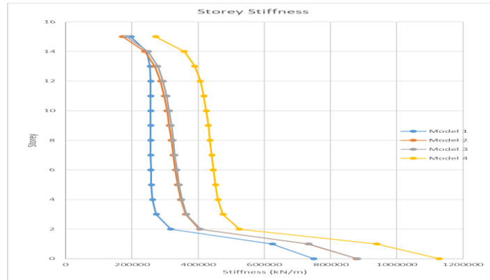
Fig 24 Graph showing Comparison of Storey Stiffness Results for Model 1(c), 2(c), 3(c) & 4(c)
