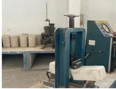
Figure 14: Flexural strength test
