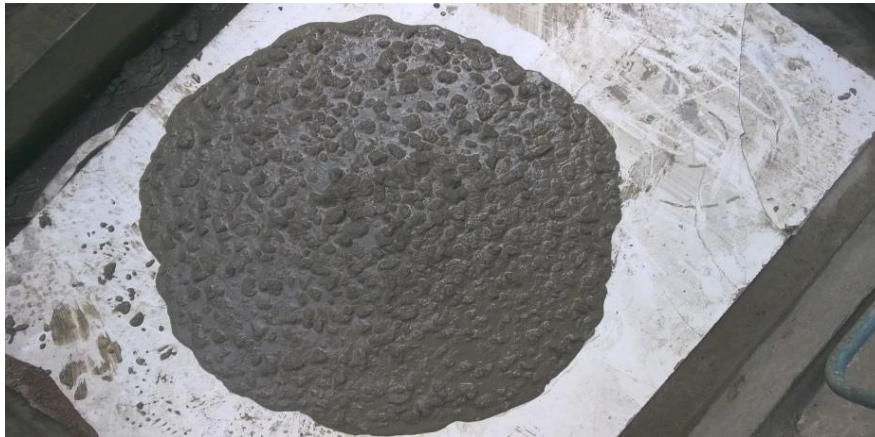
Figure 2: View of concrete spreading after slump flow test
