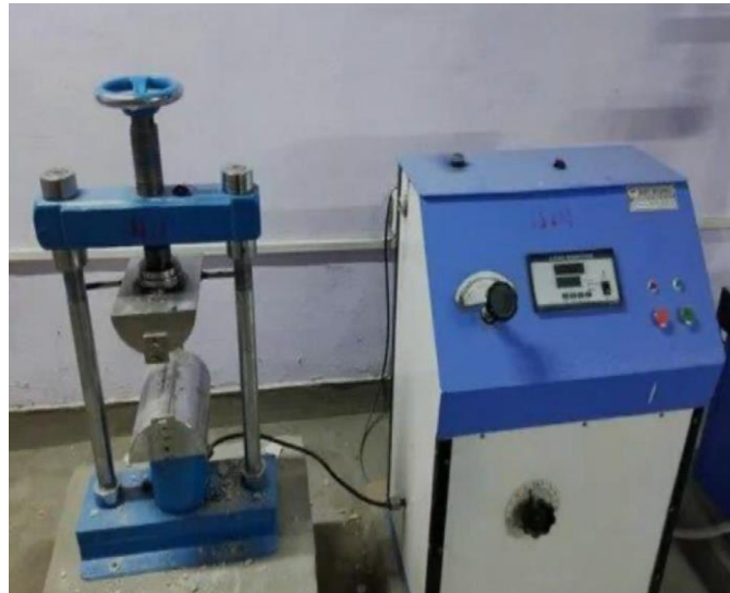
Figure 10: Split tensile strength test
