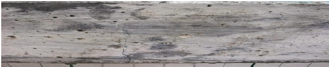
Figure 20: Crack pattern for SCC with 2% SN based CI beam
