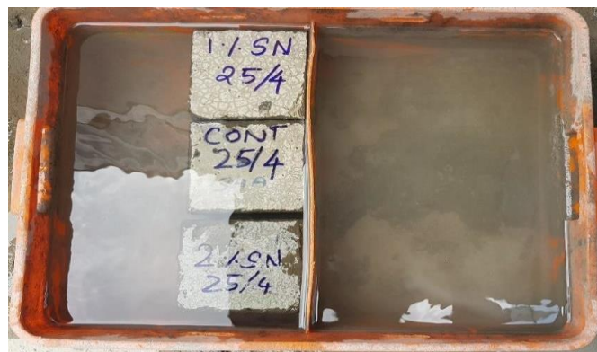
Figure 15: Chloride penetration test
