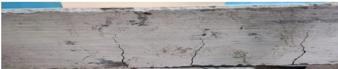
Figure 19: Crack pattern for SCC with 1% SN based CI beam
