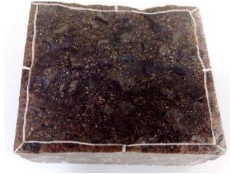
Figure 21: Tested specimen of chloride penetration test
