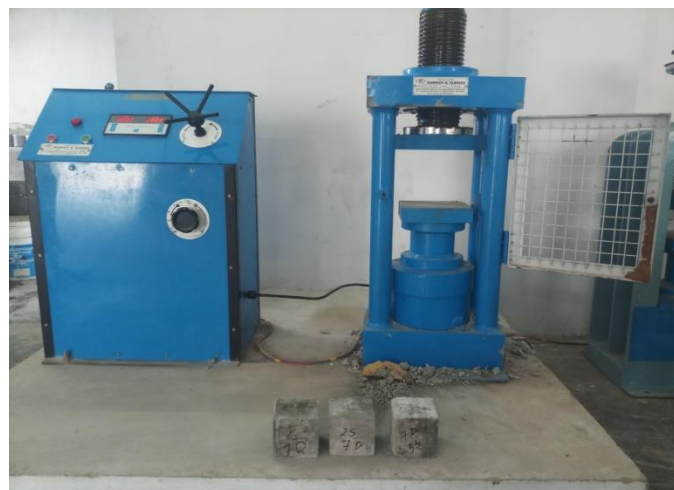
Figure 9: Compressive strength test
